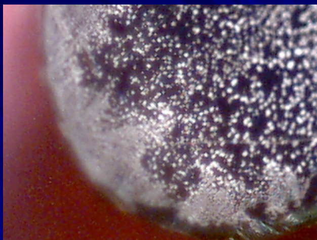
Figure 3: Dry Drop spot 0.1M CHCA in 90:10 (v/v) MeOH:H 2 O 60X magnification.
