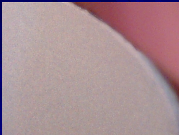
Figure 2: ES spot 0.1M CHCA in 90:10 (v/v) MeOH:H 2 O, 2 minute spray, 5670V, 60X magnification.
